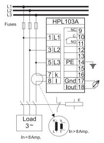
Note!!! An external current converter must always be mounted in the L3phase for correct measurement. The converter polarity is not important.
