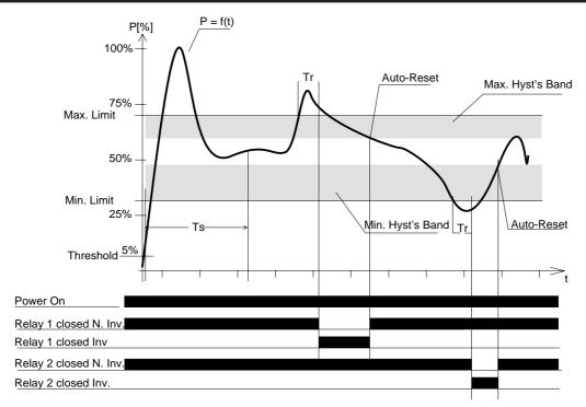
The Figure above shows a typical AC-motor power consumption curve immediately after power has been applied to the motor. The bars at the bottom of the figure indicate power applied to the unit and the position/state of the relay (On/Off). The figure shows the function of Ts, Tr and Hysteresis on the Max. 1 limit. The hysteresis
